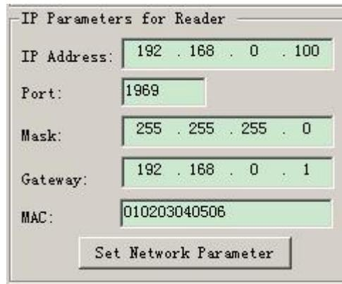
The screenshot shows a dialog box titled "IP Parameters for Reader". It contains several input fields for network configuration: IP Address (192 . 168 . 0 . 100), Port (1969), Mask (255 . 255 . 255 . 0), Gateway (192 . 168 . 0 . 1), and MAC (010203040506). A "Set Network Parameter" button is located at the bottom.
